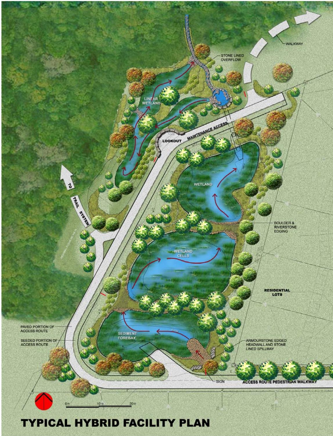
Figure 17: Demonstration Plan – Hybrid Facility
