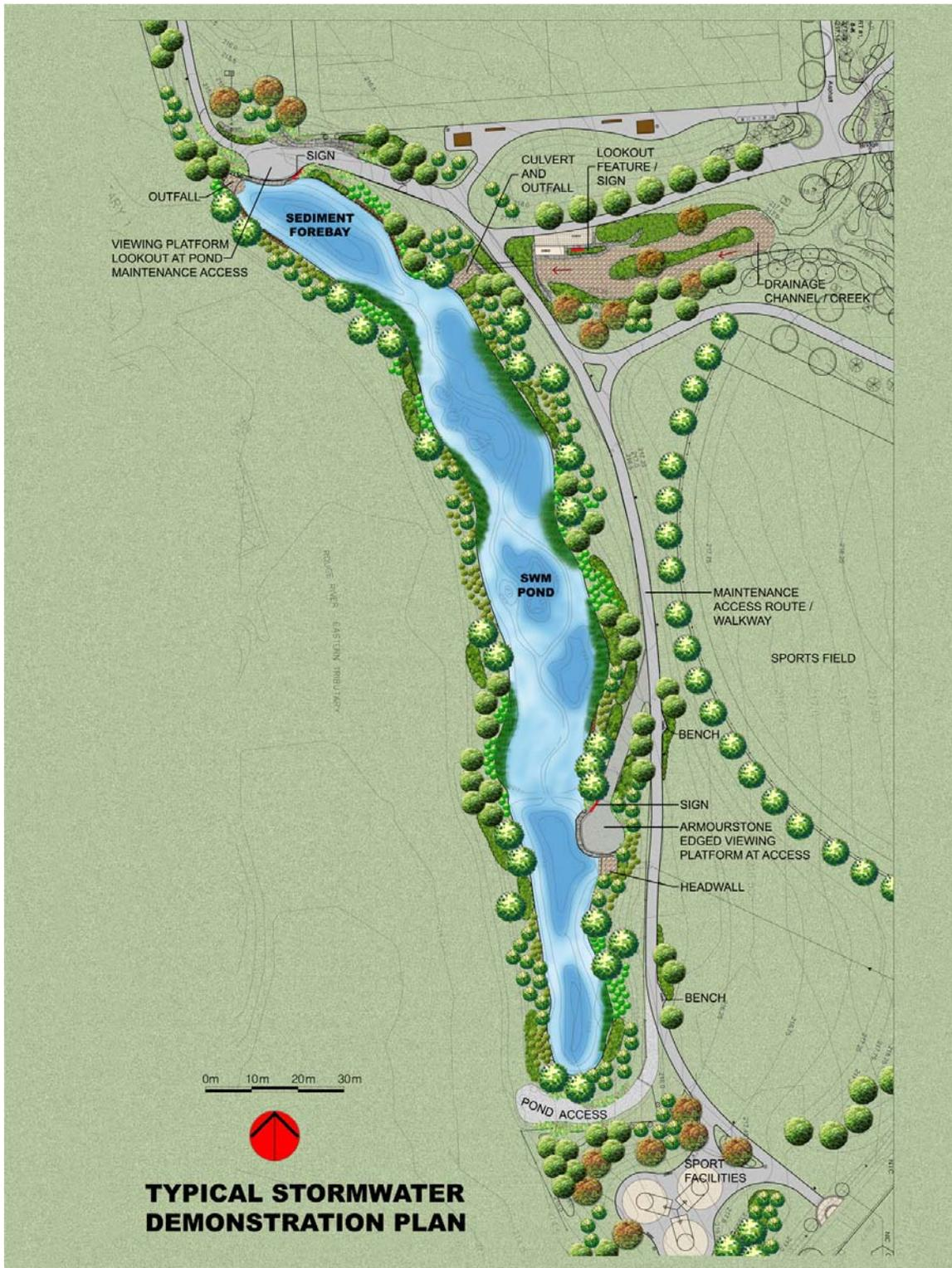
Figure 18: Demonstration Plan – Wet Pond
