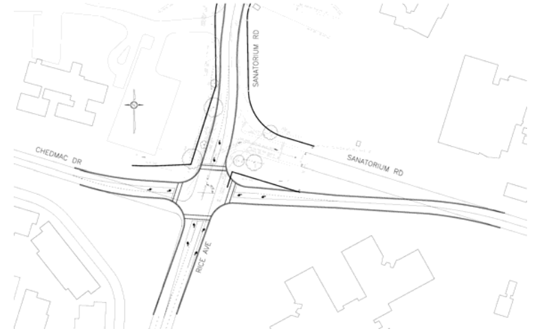
Sanatorium Road/Chedmac Drive/Rice Avenue realigned for traffic signals.
