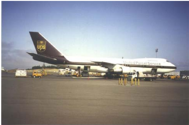
Existing tenants must be able to upgrade capacity to Code E aircraft like this UPS B747. (Source: LPS AVIA)
