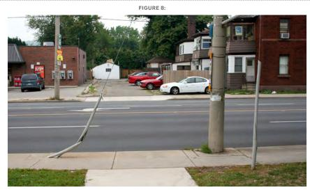
A non-accessible bus stop with a utility guy wire obstructing the landing pad area, without any reflective sheath
