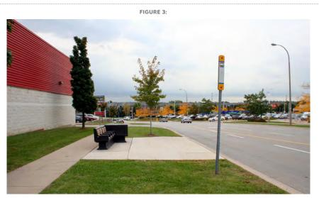
Landing pad long and deep enough to deploy the ramps and have space to manoeuvre
