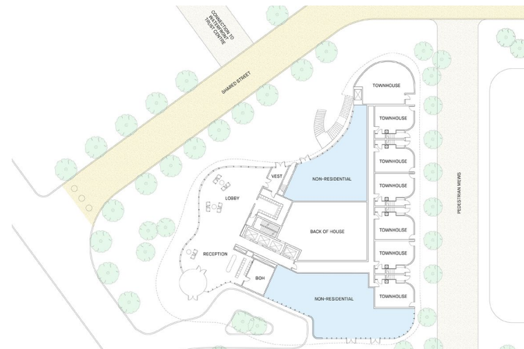
Ground Floor Plan (KPMB Architects) illustrating the interface between the feature staircase and non-residential spaces at-grade
