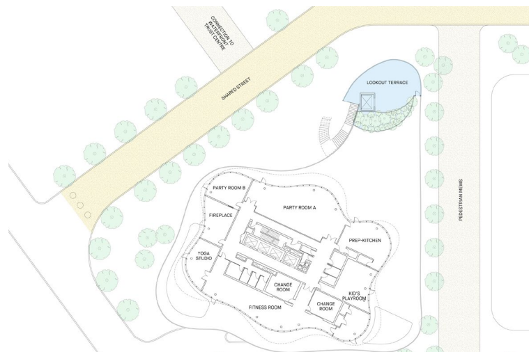
Podium Roof Plan (KPMB Architects) illustrating the location of the lookout terrace and landscape buffer
