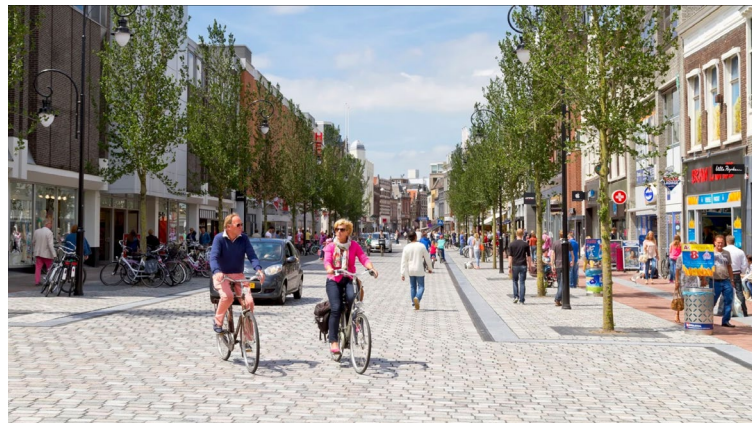
Example of a ‘woonerf’ or shared-street in the Netherlands, with spaces for active transportation and pedestrians, as well as limited vehicle access
