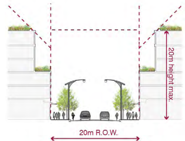
Maximum allowable height is determined by the width of the public right-of-way (all references to the R.O.W. or R.O.W. widths, denotes the public R.O.W.).
