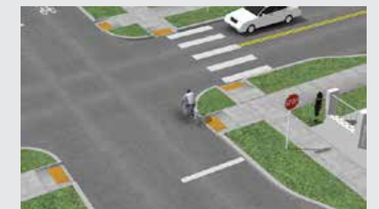
The Breadalbane and Pearl-Kent neighbourhood greenway installations will include measures such as wayfinding and directional signage (top) to help navigation and curb extensions at intersections (bottom) to help manage automobile speeds along the corridors.
