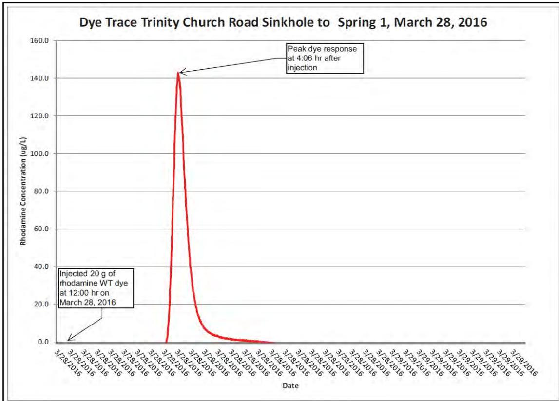
Figure 3.10: Results of Sinkhole Dye Trace
