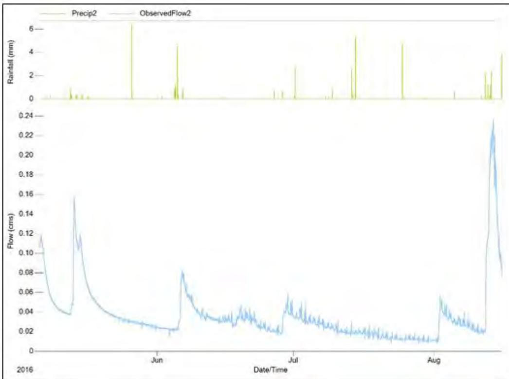
Figure 3.31: Observed Rainfall and Estimated Flow at Site 2 - Sinkhole Creek
