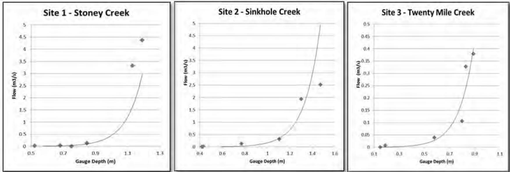
Figure 3.29: Stream Gauge Rating Curve Development
