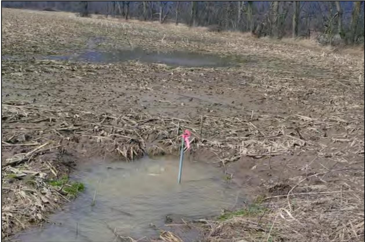
Figure 3.15: Groundwater bubbling up at GW3
