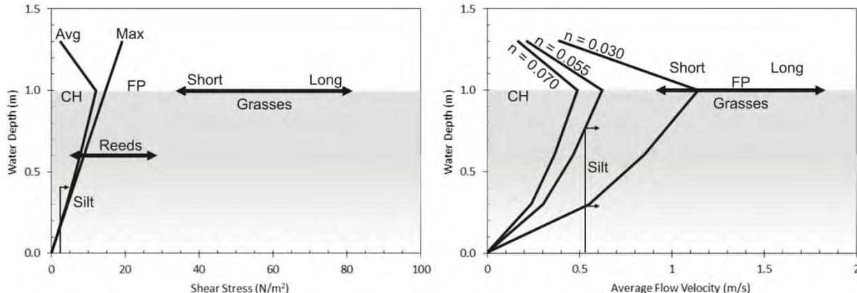
Figure 3.27: Simplified estimates of erosion thresholds for vegetation-dominated ditches
