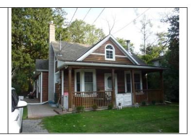
Foundation: Construction Material: (Wood-frame) Cladding: Siding; Shingles (in gable) Roof Type: Gable Roof Material: Asphalt
