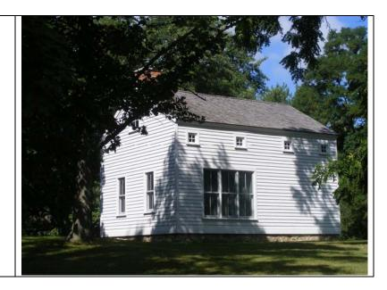
Foundation: Stone Construction Material: (Wood-frame) Cladding: Siding (horizontal) Roof Type: Gable Roof Material: Asphalt
