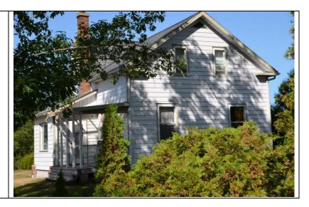
Foundation: Construction Material: (Wood-frame) Cladding: Siding (horizontal) Roof Type: Gable (Side) Roof Material: Asphalt
