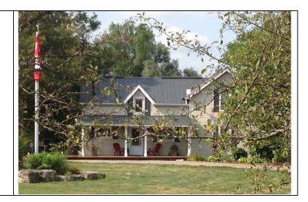
Foundation: Construction Material: (Wood-frame) Cladding: Siding (horizontal) Roof Type: Gable (Cross) Roof Material: Metal (standing seam)
