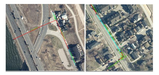
• Pipe placement inconsistencies at Pipe 55427 in 2021-01 data and 2021-05 data
