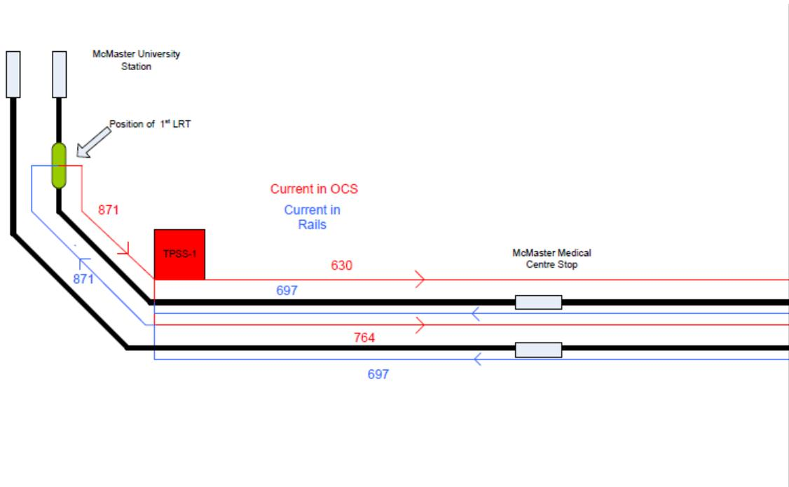
Figure 9: Current Magnitude and Direction, Outage at 2<sup>nd</sup> Substation
