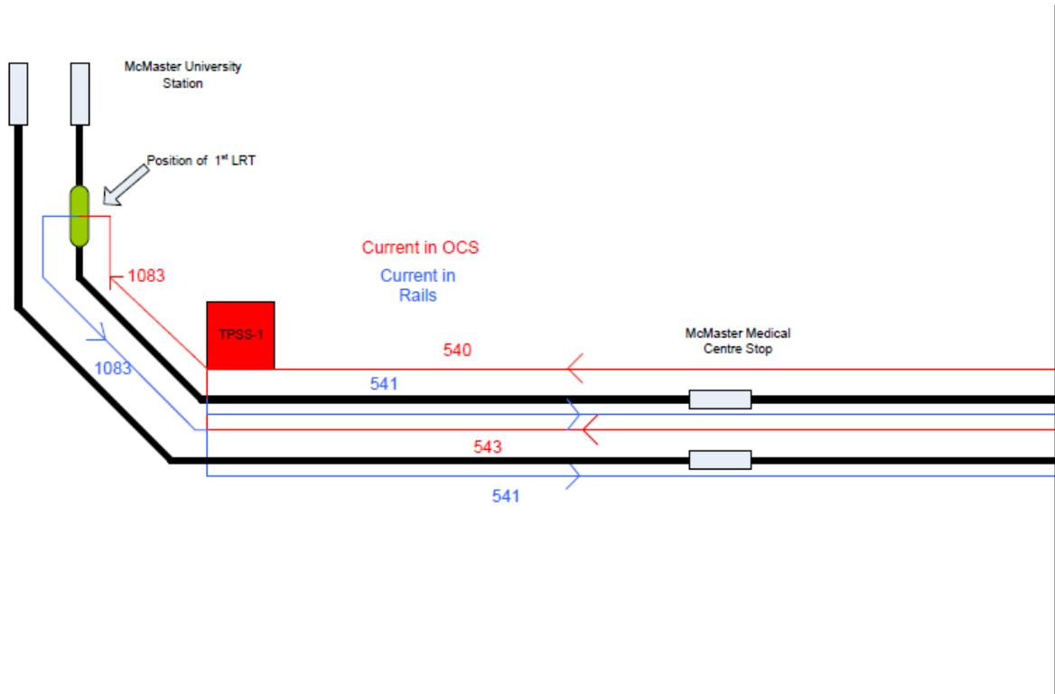
**Figure 7: Current Magnitude and Direction, Outage at 1<sup>st</sup> Substation**
