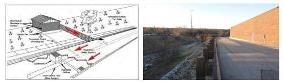
(From L to R: Conceptual Curb and Gutter, Concrete Lined Surface Channel)
