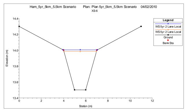
**Figure 4.20** – Surface water elevation of the various runoff flow accumulation from 5km and 5.5km of 2 lane local road.
