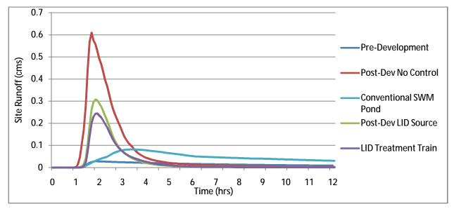
Figure 4.17: Runoff Characteristics of a 25 mm 6hr Event for a 20ha Site Plan Test Case
