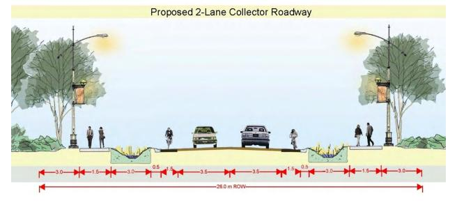
Figure 3.2: Proposed -2Lane Arterial Roadway with 3m allowance for LID conveyance Controls
