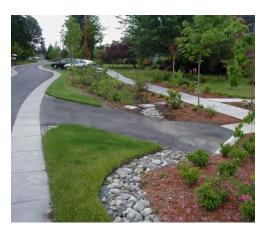
Combining filter strips with other best management practices is highly recommended. They can also provide a convenient area for snow storage and treatment, and are particularly valuable due to their capacity for melt water infiltration. Because filter strip designs include few pipes or other structures, physical changes to the practice are not needed for wintertime operation. Furthermore, many of the pollutants in the snowpack can be treated through infiltration where groundwater
