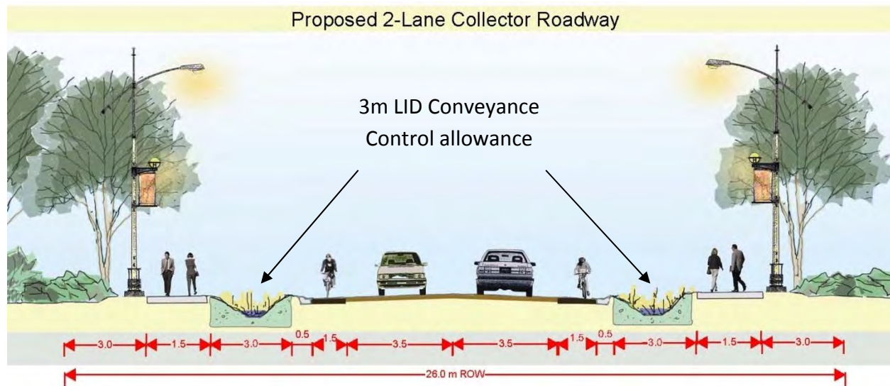
Figure 3.4.1: Example AEGD Cross section with 3m allowance for LID conveyance Controls
