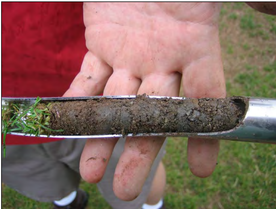
Figure 4. Soil core sample from Heritage Green field showing irregularity of rootzone material.
