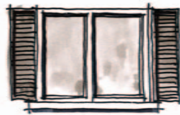
The shutters on this window reflect a lack of proportion.
