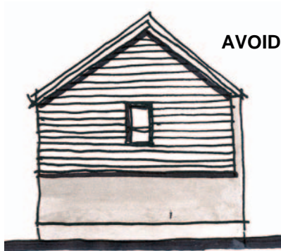
A 50/50 split of materials is not acceptable where the building is visible from the street.
