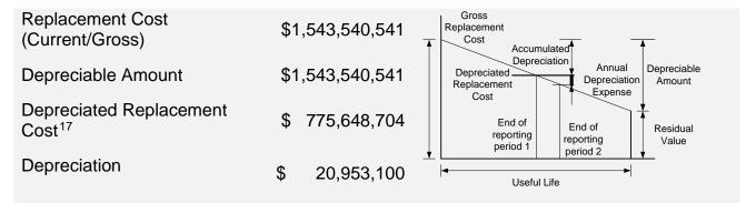
The current replacement cost is the most common valuation approach for specialized infrastructure assets such as engineered structures. The methodology includes establishing a comprehensive asset registry, assessing replacement costs (based on market pricing for the modern equivalent assets) and useful lives, determining the appropriate depreciation method, testing for impairments, and determining remaining useful life.
