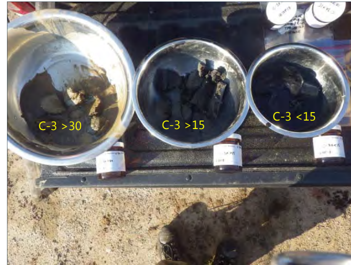
C-3 core strata prior to homogenizing.
