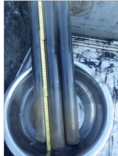
Example of core tubes with sample from C-3.
