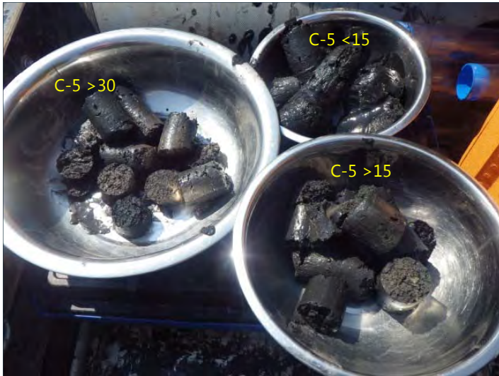
C-5 core strata prior to homogenizing.
