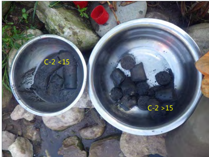
C-2 core strata prior to homogenizing.
