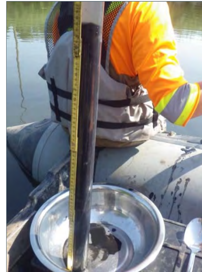
Example of a core tube with sample from replicate near west bank.
