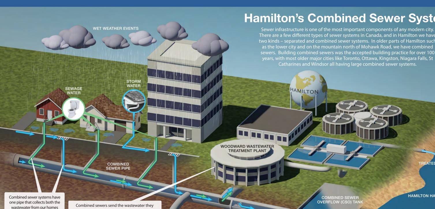
collect to our wastewater treatment plant where and businesses, and stormwater it is cleaned and released into Hamilton Harbour. from rain or melted snow.
