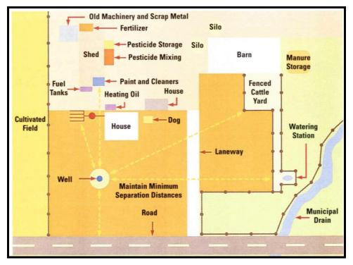
Figure 1. Locating a potable water well supply
