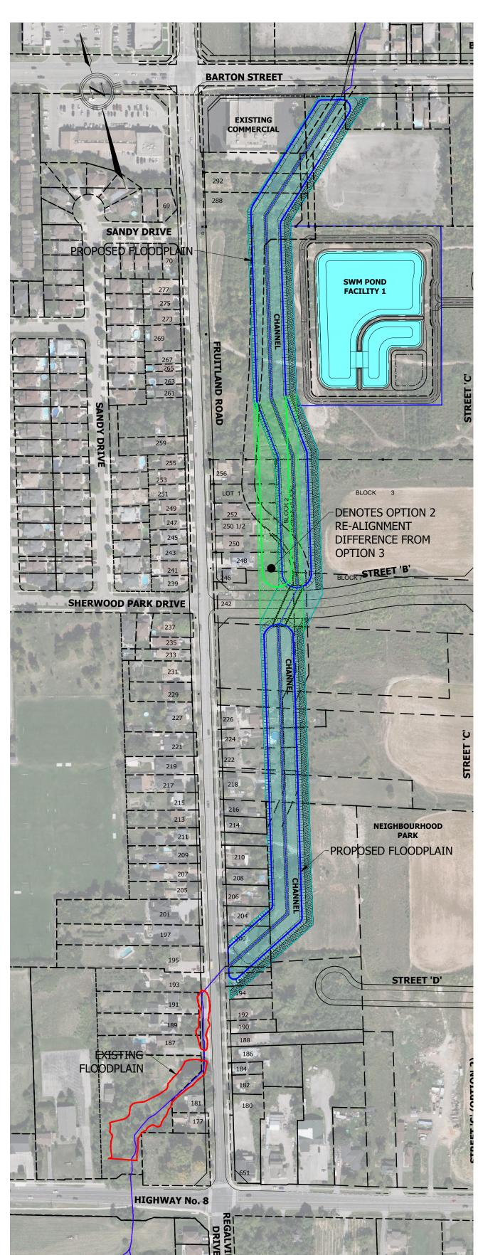
THIS DIAGRAM ILLUSTRATES TWO POSSIBLE ALIGNMENTS FOR PROVIDING AN ENHANCED NATURAL CHANNEL DESIGN.
