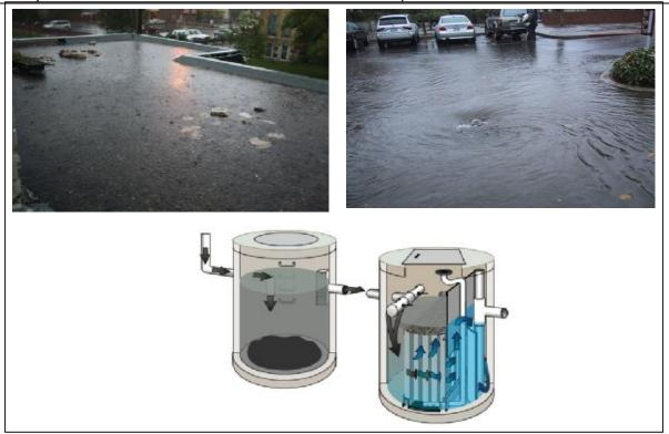
Figure 7.8.2: Traditional Source Controls (Clockwise, from top left: Rooftop Storage, Parking Lot Storage, Oil-Grit Separator)
