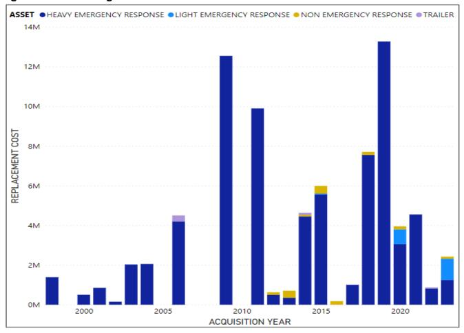
Per *Figure 4*, there are acquisition spikes in 2009, 2011, and 2019 for heavy emergency response vehicles (i.e., rescue, pumper, engine, ladder, and tanker apparatus). Since these vehicles have an estimated service life Estimated Service Life of 20 years, there will be spikes in renewals in 2029, 2031 and 2039 as discussed in **Section 8.3.**
