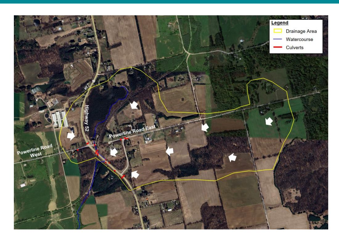
Existing drainage is conveyed through roadside ditches, and crossing and entrance culverts to a GRCA regulated watercourse which drains to the Big Creek Headwaters Wetland Complex
