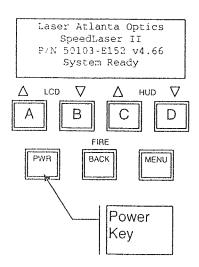
When the SpeedLaser is first turned ON, it automatically runs the self-test function. To capture a speed, simply follow the procedure below.
