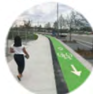
2.0m Sidewalk & 2.0m Cycle Track on Both Sides of the Road (+0.6m Buffer)
