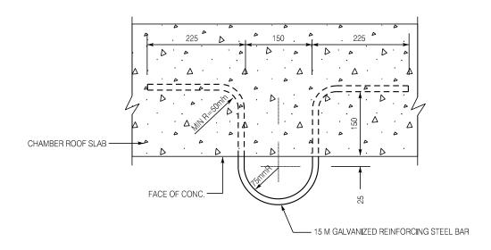
LIFTING HOOK TO BE LOCATED DIRECTLY ABOVE VALVES, ACCESS MANHOLES, ETC. AS INDICATED ON VALVE CHAMBER DRAWINGS
