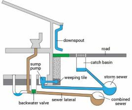
Best Practice recommends that downspouts discharge to the ground surface, and the Foundation Drain should discharge to the ground if the soil conditions permit or connect to the Storm Sewer if available
