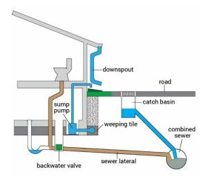
Best Practice recommends that downspouts discharge to the ground surface, and the Foundation Drain should discharge to the ground if the soil conditions permit or connect to the Storm Sewer if available
