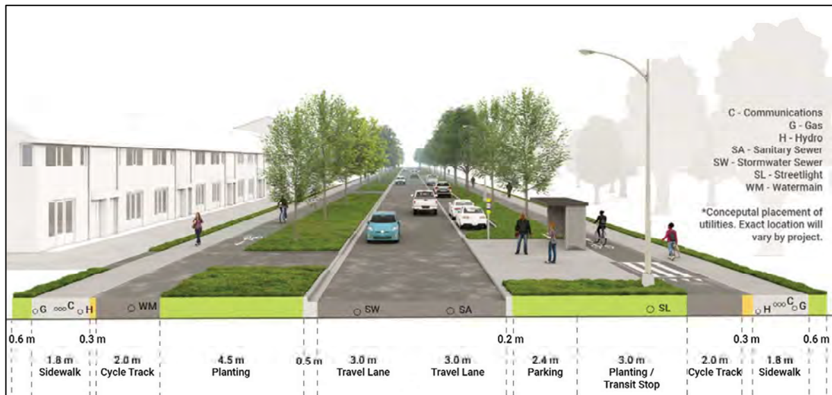
Figure 7.3) Typical Connector Cross-Section
