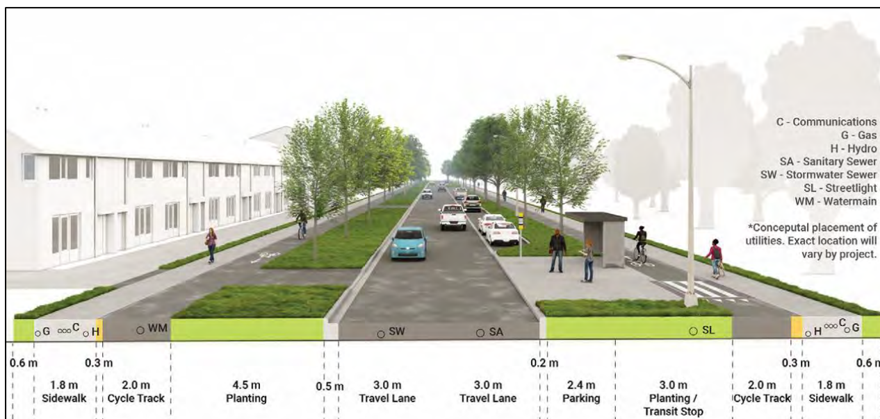
Figure 7.3) Typical Connector Cross-Section
