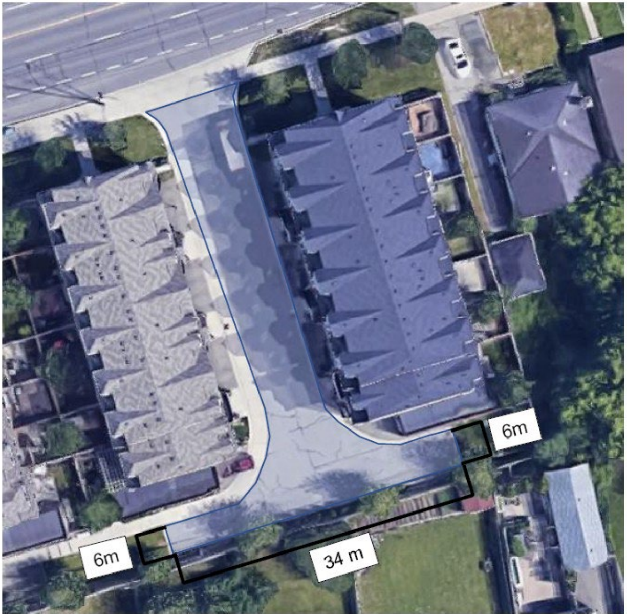
Figure 6. Aerial image of an existing Development in Hamilton featuring an acceptable T-Turnaround.
