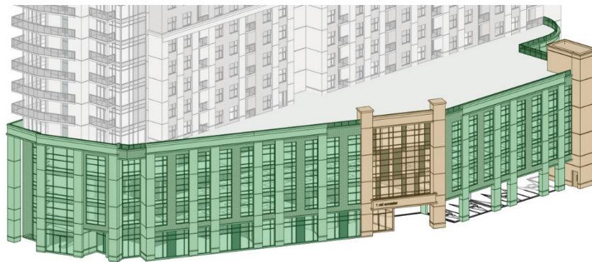
Figure 16 - Horizontal Break-up of Podium Massing
