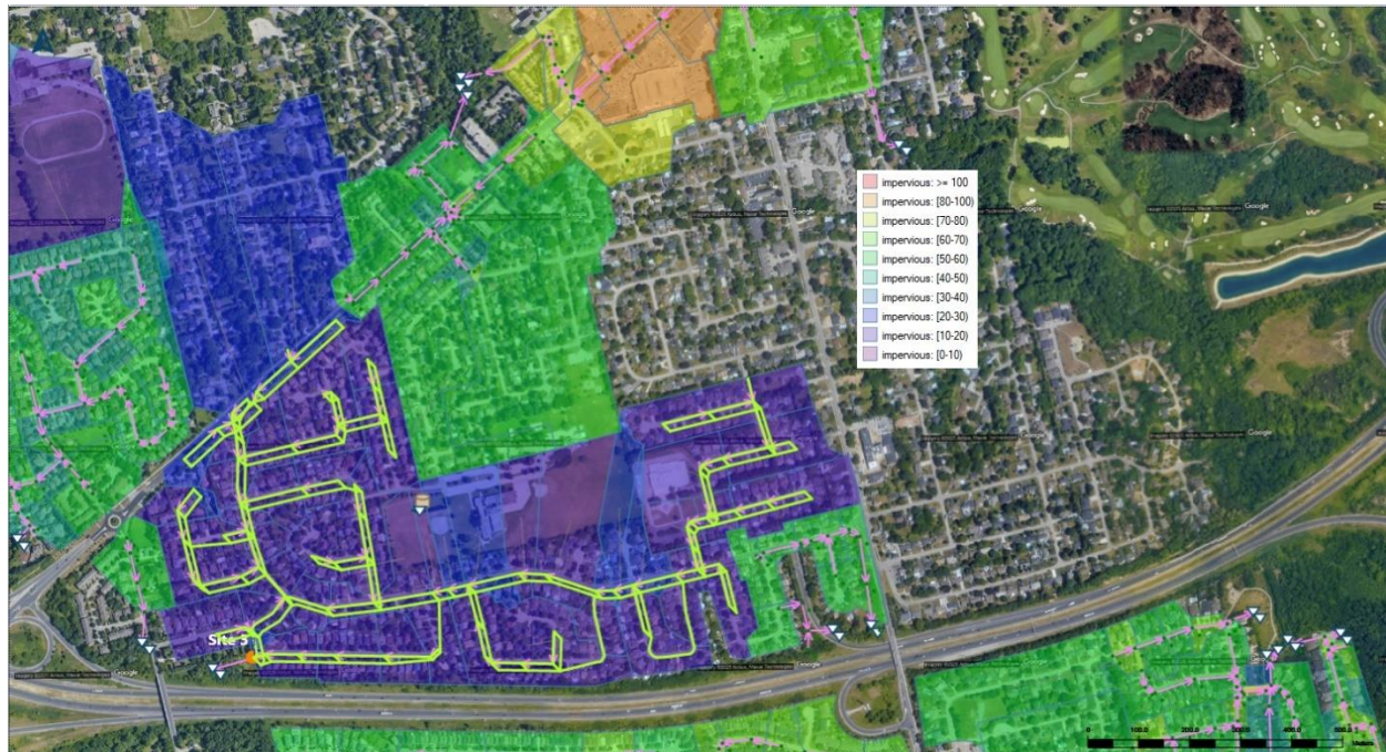
Figure 4.2.2: Example map of inconsistent imperviousness values for catchments in the Ancaster model
