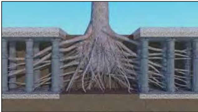
Figure 5-3: Soil Retention/Tree Planter Cell Cross Section ( info.cambrianrisevt.com , 2020)
