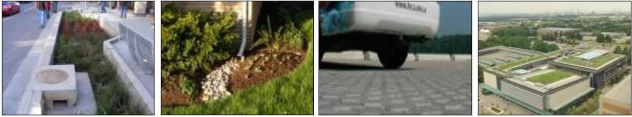
**Figure 7.8.3: Example LID Source Controls (from L to R: Bioretention, Downspout Disconnection, Permeable Pavement, Green Roofs)**
