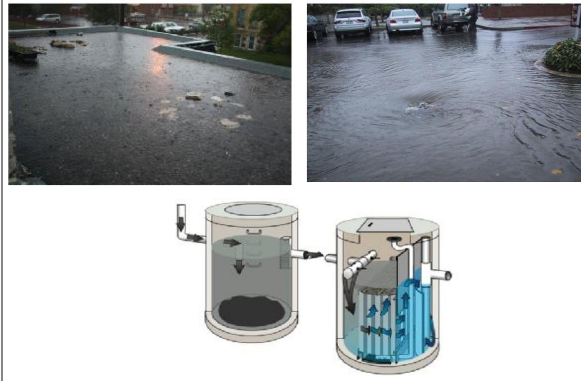
**Figure 7.8.2: Traditional Source Controls (Clockwise, from top left: Rooftop Storage, Parking Lot Storage, Oil-Grit Separator)**
