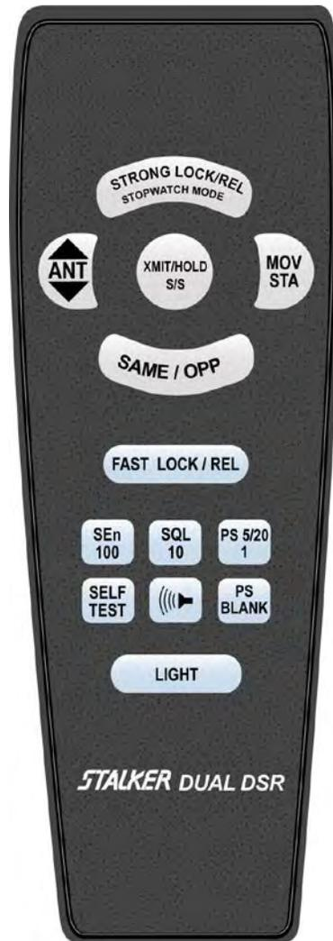
The Remote Control can be operated in wired mode by connecting a standard RJ-11 modular telephone handset cord (P.N. 155-2213-00 or Radio Shack #279-312). The cord is connected to the remote and radar unit, and battery removed for wired operation.
