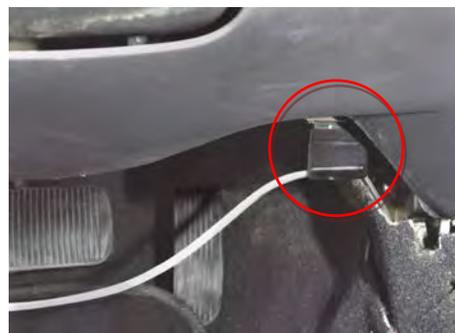
The CAN/VSS Adapter is Stalker’s preferred method for automating the radar’s patrol speed acquisition as well as transitioning back and forth between stationary to moving modes.
